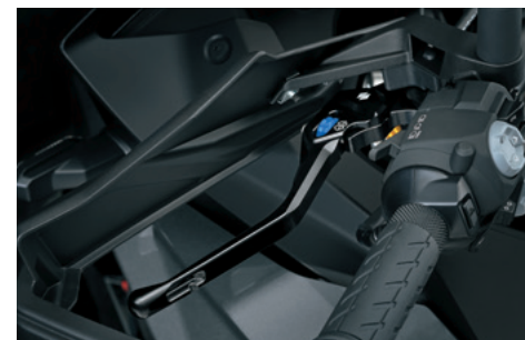
Billet Clutch Lever (Anodized) 57600-48810-000 Machined from high-end billet aluminum, decorated with GSX-S logo (in front) and Suzuki "S" logo. These black anodized levers provide a more sporty look to the vehicle. There are two different colors (blue and red) for the lever adjuster that comes along with this item. You can choose which one to use at your preference.
