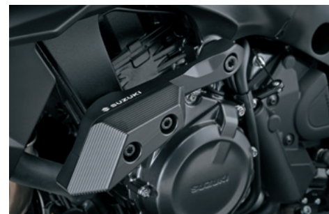
Frame Slider 41900-48810-000 Helps mitigate damage, made of aluminum and POM (polyacetal).
