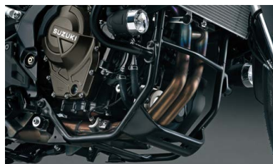
Accessory Bar Tube 41100-25810-000 Required for installing accessory bar (94200-25810-000), aluminum skid plate (p/n 42500-25830-000), or under cover (p/n 94400-25830-000).
