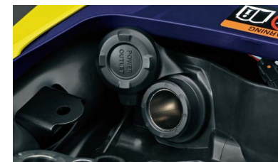
DC Socket 38800-31810-000 Gives option to customers for usage of electric devices. To be installed underneath seat.
